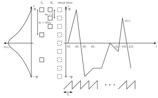
Fig. 2. Random PCM properties with the PCM PDF on left side and the uncorrelated phase center positions at the right side.
