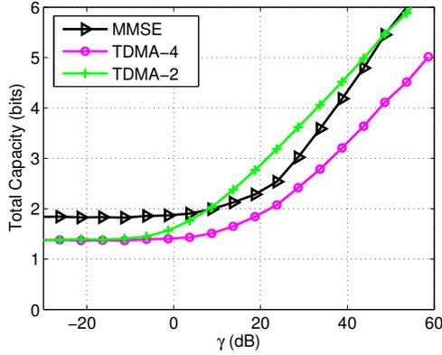
Fig. 4. Total capacity per time-slot with  $\eta = 17dB$ .
