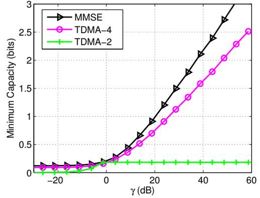
Fig. 3. Minimum capacity per time-slot with  $\eta = -3dB$ .
