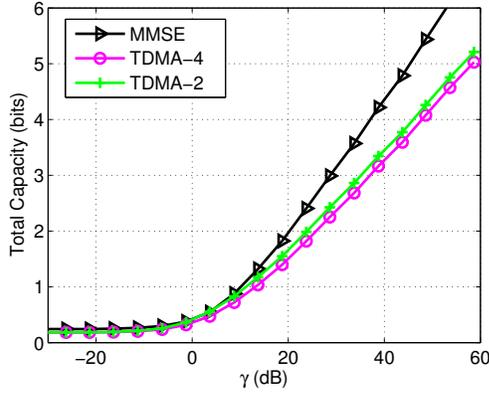
Fig. 2. Total capacity per time-slot with  $\eta = -3dB$ .
