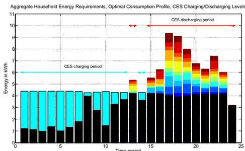
**Fig. 2.** Energy visualization bar graph. (cyan+black) Optimal consumption profile of all households, (black+multi-colour) Aggregate energy requirements of all households, (cyan+multi-colour) CES batteries' charging and discharging profiles, (multi-colour) Amount of stored energy sold to all households along with the individual household allocation.
