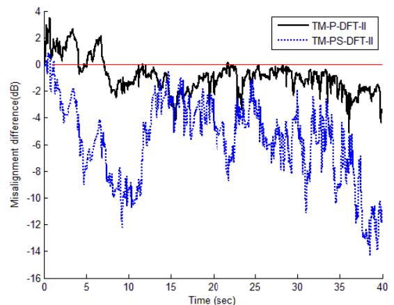
**Fig. 8.** Misalignment difference for 8 and 16 subbands respectively. Other conditions are those from Fig. 4.
