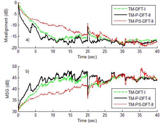
**Fig. 6.** (a) Misalignment and (b) MSG curves with speech input, probe injection and feedback path variation at 20 seconds.
