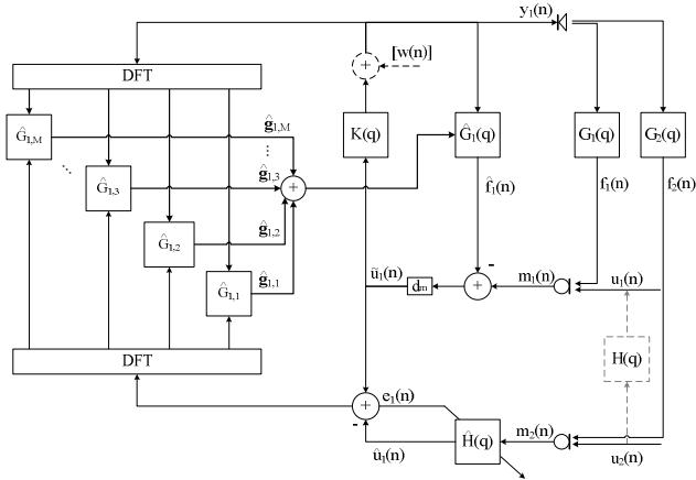
**Fig. 3.** TM Type II block diagram without subband decomposition of  $\hat{H}(q)$ .
