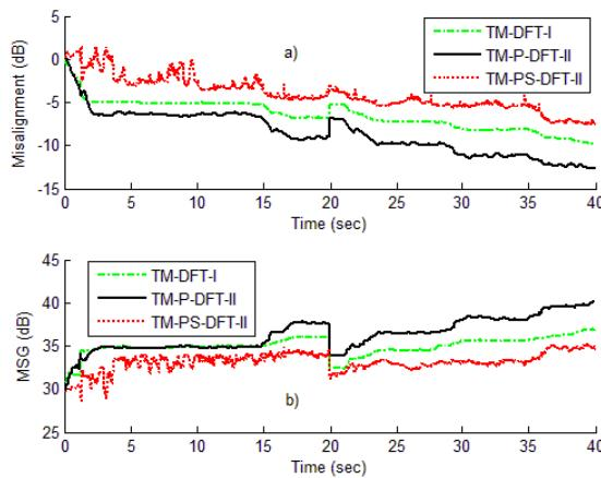
**Fig. 5.** (a) Misalignment and (b) MSG curves with music input, feedback path variation at 20 seconds.
