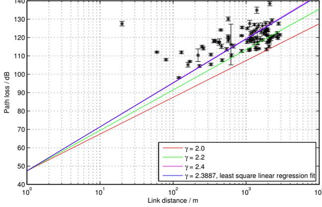
**Fig. 5.** Path loss  $L$  versus link distance  $d$  measured on Ttree, with linear approximations and a least squares fit.
