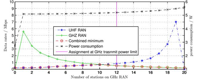
**Fig. 7.** Individual station capacity on each RAN and base station power consumption given possible valid RAN assignments.
