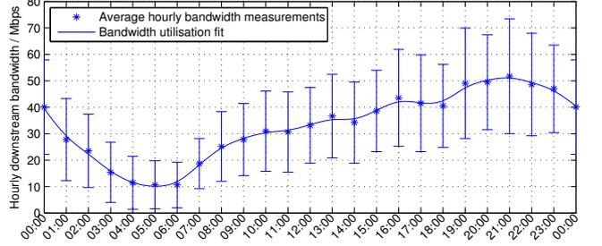
**Fig. 8.** Mean downlink bandwidth of Tiree network and fitted model.
