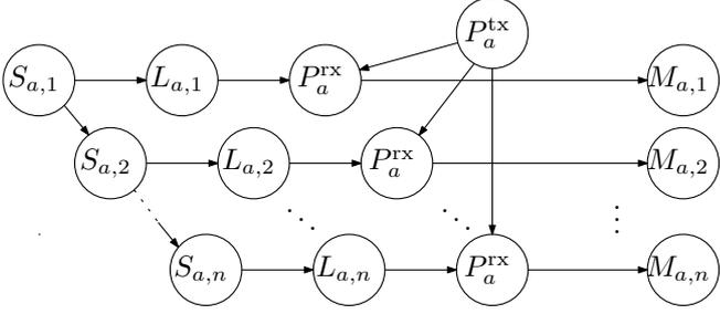
**Fig. 2.** BBN describing dependencies of distance, path loss, receive power and data rate.
