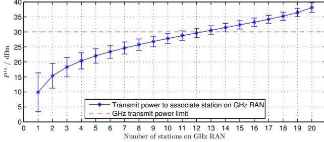
**Fig. 6.** Mean beliefs of  $\mathcal{P}_g^{\text{tx}}$  with standard deviation after BBN convergence to associate stations with the GHz RAN.
