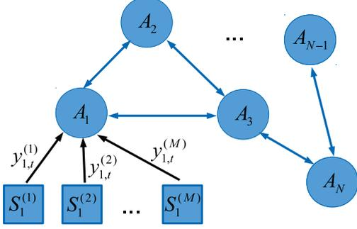
**Fig. 1.** A schematic diagram of a distributed system, where  $A_n$  denotes the  $n$ th agent,  $S_n^{(m)}$  represents the  $m$ th sensor of agent  $A_n$ , and  $y_{n,t}^{(m)}$  denotes the measurements provided from  $S_n^{(m)}$  to  $A_n$  at time instant  $t$ .
