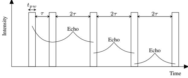
Fig. 1. The NQR signal formed using a PSL sequence.
