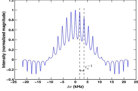
**Fig. 2.** Theoretical model of the NQR signal magnitude as a function of the frequency offset,  $\Delta\omega = 2\pi\Delta\nu$ , for a PSL sequence, using the 3.6 MHz spectral line of sodium nitrate as the sample model.
