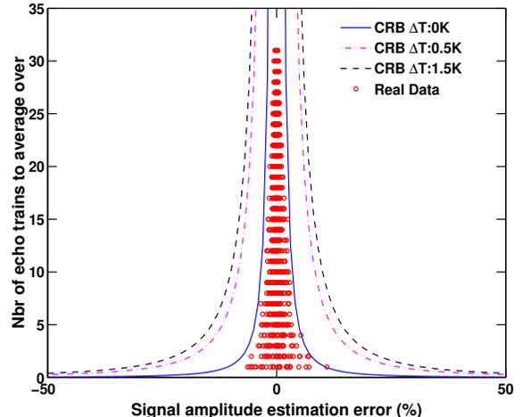
**Fig. 4.** The 99% estimation accuracy as determined using the CRB of the NQR signal intensity at different offset frequencies. The theoretical bounds are compared with NQR measurements on sodium nitrate, for the 3.6 MHz spectral line.
