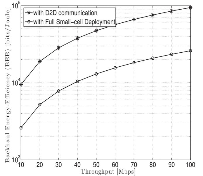
Figure 3. Backhaul energy-efficiency comparison of D2D communication against full small-cell deployment for fixed macrocell radius of  $R_m = 500$  m.
