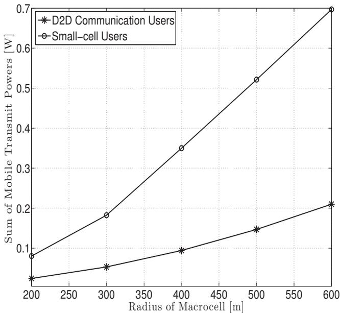
Figure 4. Tier 2 uplink sum transmit power comparison of D2D communication against full small-cell deployment.
