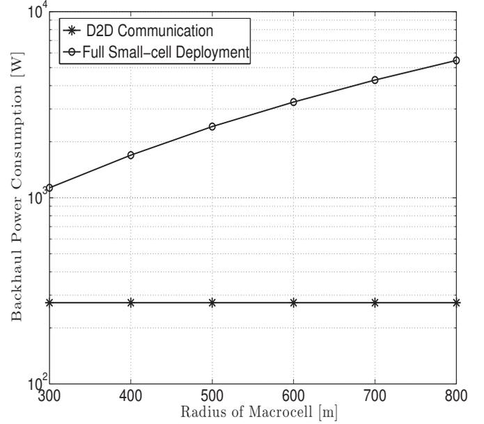
Figure 2. Backhaul power consumption comparison of the network with D2D communication against full small-cell deployment.
