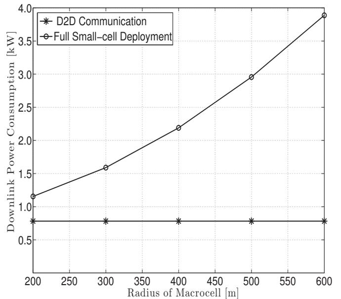
Figure 5. Downlink power consumption comparison of D2D communication against full small-cell deployment.
