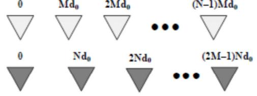
Fig. 2. Extended co-prime array configuration
