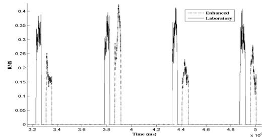
**Fig. 9.** RMS waveforms of enhanced and reference EMG signals.
