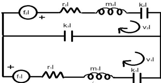
Fig. 2. Electromechanical equivalent circuit of vocal folds.
