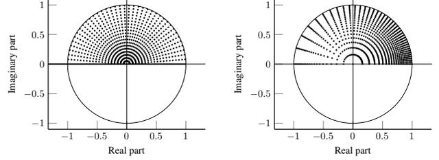
**Fig. 2:** Pole grids with uniform (left) and logarithmic (right) radius and angle distributions.
