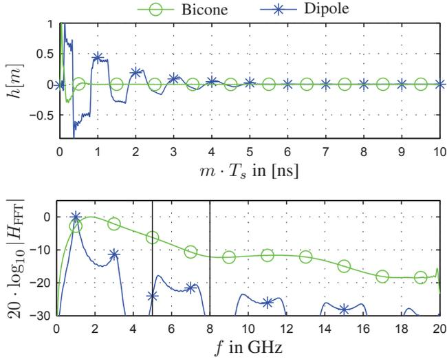
**Fig. 5.** Normalized impulse responses (top) and frequency response magnitudes (bottom) of Dipole and Biconical antennas.  $f_l$  and  $f_u$  are indicated by two solid black vertical lines.
