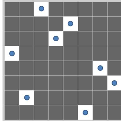
**Fig. 1.** A Costas array of size  $8 \times 8$ .
