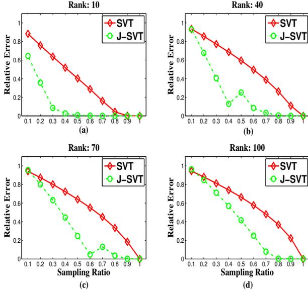
**Fig. 1.** Relative error as a function of sampling ratio. The size of dictionary  $\mathcal{G}$  is  $300 \times 1500$ . The rank of matrix  $L$  is: (a) 10, (b) 40, (c) 70 and (d) 100.
