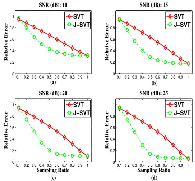
**Fig. 3.** Relative error as a function of sampling ratio. The size of dictionary  $\mathcal{G}$  is  $300 \times 1500$  and the rank of matrix  $L$  is 50. The SNR level is set to: (a) 10 dB, (b) 15 dB, (c) 20 dB and (d) 25 dB.
