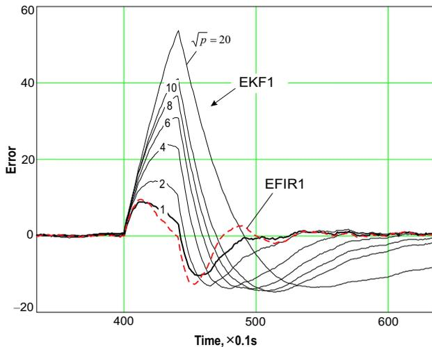
Figure 4: Effect of the temporary model uncertainty occurred from  $n = 400$  to  $n = 440$  on the estimation errors with  $p \geq 1$ .
