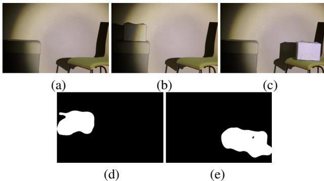
**Fig. 7.** Input images and masks of the experiment (Figure 6): (a) background image, (b) reference image, (c) target image, (d) mask of current image, (e) mask of target image.
