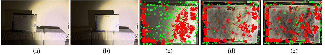
**Fig. 5.** Results of lighting effect removal: (a) reference frame, (b) target frame, (c) conventional method [4], (d) non-removal, (e) our method. The trackable points are red circles, while the failed points are green x-marks.
