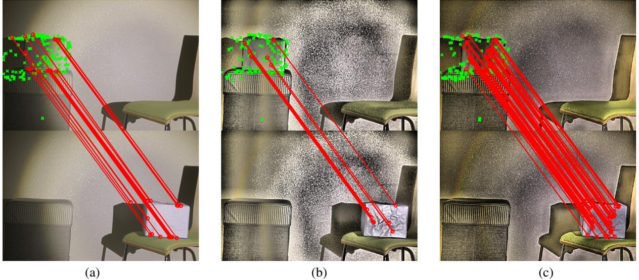
**Fig. 6.** Comparison of the results: (a) Reinhard [4], (b) Reinhard[4] + CLAHE, (c) Our method. The red circles denote valid feature points and green x-marks indicate failed feature points.
