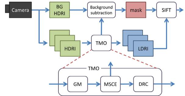
**Fig. 1.** Our assumed HDR camera surveillance system: (BG HDRI) BackGround HDR Image, (TMO) Tone-Mapping Operator, (GM) Gamma Mapping, (MSCE) Multi-Scale Contrast Enhancement, (DRC) Dynamic Range Compression.
