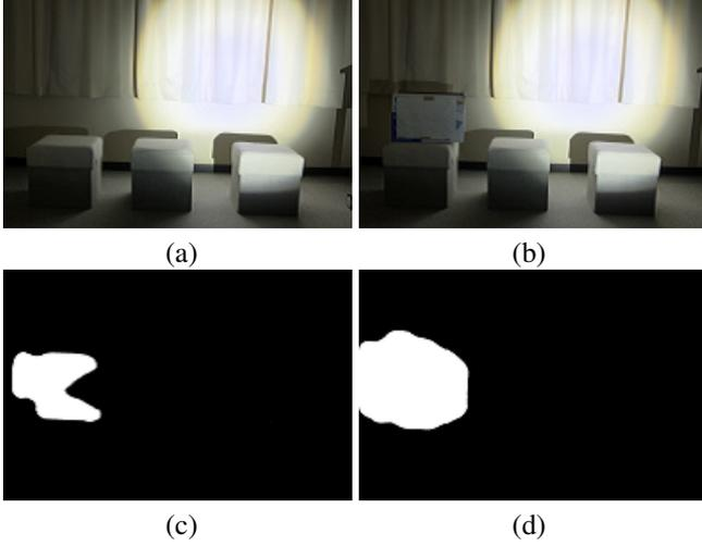
**Fig. 3.** Estimation results for a moving object: (a) background frame, (b) target frame, (c) conventional method with adapted threshold, (d) our method.
