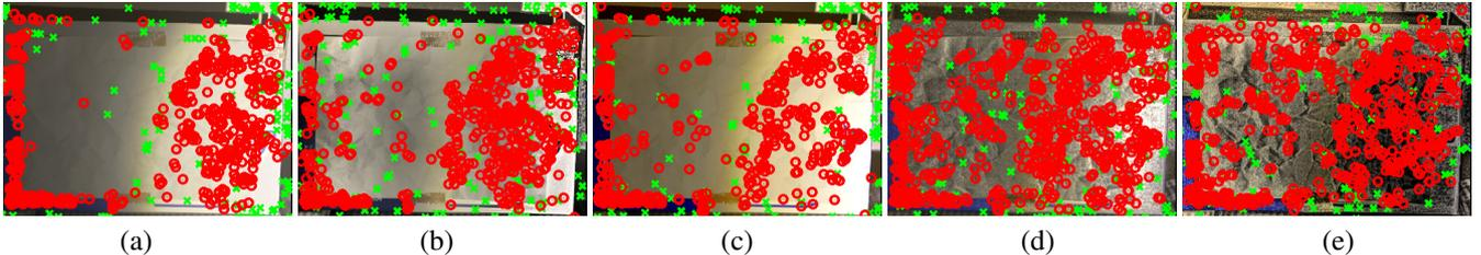
**Fig. 9.** Results (reference:"box3", target:"box4"): (a) Reinhard[4], (b) Reinhard + CLAHE, (c) Subband[5], (d) Local Laplacian[6], (e) Our method. The trackable points are red circles, while the failed points are green x-marks.
