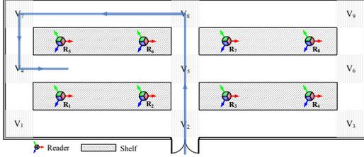
**Fig. 1.** The RFID system in the considered warehouse layout.
