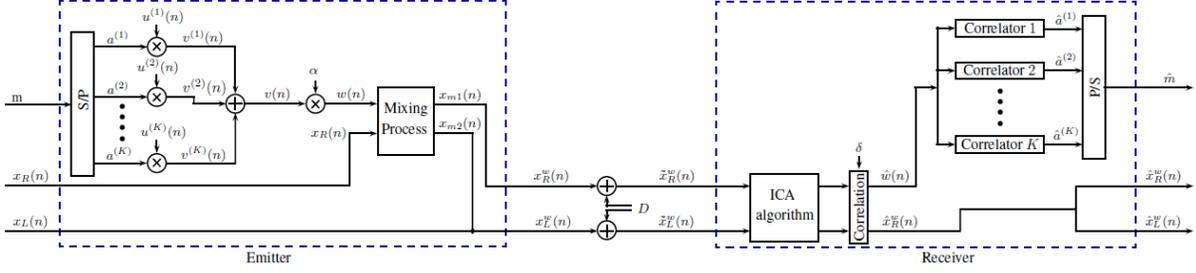
**Fig. 1.** The proposed CDMA-ICA two-channel audio watermarking scheme.
