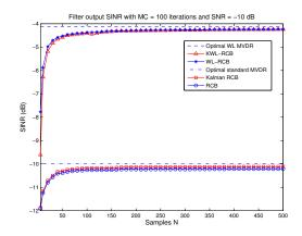
Fig. 2. Output SINR as a function of sample length for noncircular BPSK signals with SNR = -10 dB. Red triangles and blue asterisks are robust WL beamformers and perform equally, while the former, the proposed Kalman implementation, has reduced complexity.
