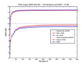
Fig. 1. Output SINR as a function of sample length for noncircular BPSK signals with SNR = 10 dB. Red triangles and blue asterisks are robust WL beamformers and perform equally, while the former, the proposed Kalman implementation, has reduced complexity.
