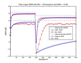
Fig. 3. Output SINR as a function of sample length for nonstationary BPSK signals at SNR = 10 dB. At N = 200the arrival direction of the interference change and the beamformers tries to adjust correspondingly. The figure shows how Kalman based beamformers deals with non-stationarity faster than SOCP based beamformers.
