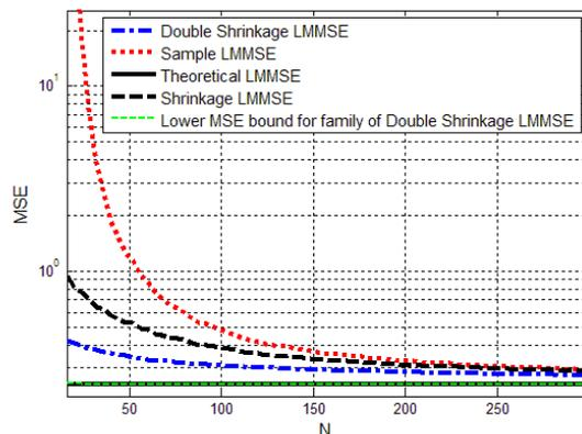
**Fig. 1:** Performance comparison between proposed double shrinkage LMMSE (14), theoretical LMMSE estimator (3), sample LMMSE (4) and shrinkage LMMSE (9).
