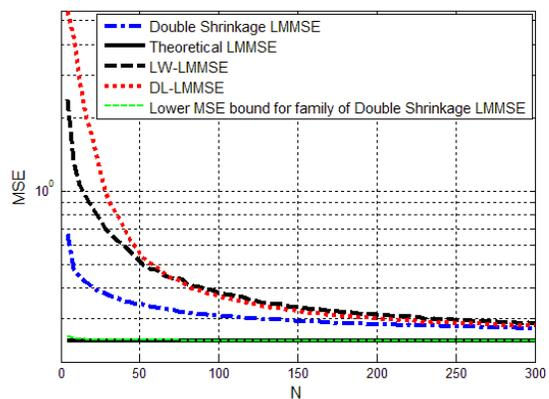
**Fig. 2:** Performance comparison between proposed double shrinkage LMMSE (14), theoretical LMMSE estimator (3), LW-LMMSE (6) and DL-LMMSE (5).
