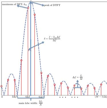
**Fig. 1.** DTFT (dash line) and  $M$ -point DFT of an  $N$ -point single-tone signal  $x(t) = Ae^{j(2\pi ft + \phi)}$  with sampling frequency  $f_s$ .
