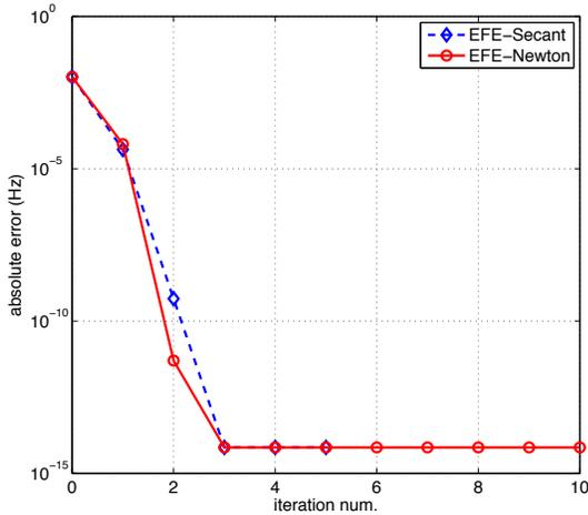
**Fig. 2.** Noiseless absolute bias comparisons between EFE-Newton and EFE-Secant on Candan11 with different iteration number. The true frequency  $f = 55$  Hz.
