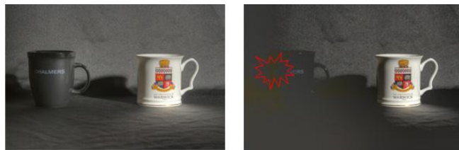
Figure 2: Tone mapped image of a scene after being captured with (left) 20 f-stops (right) 16 f-stops. Missing detail indicated in red [1].
