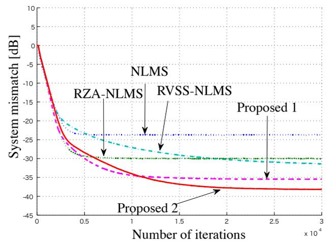
**Fig. 2.** Comparison of system mismatch (under impulsive noise). Comparison of system mismatch (no impulsive noise).
