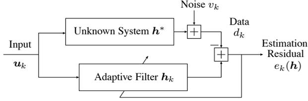
Fig. 1. Adaptive filtering scheme.
