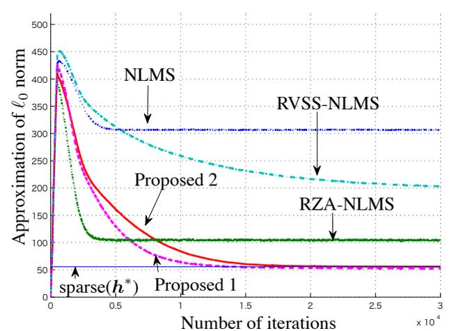
**Fig. 3.** Comparison of  $\text{sparse}(h_k)$  (under impulsive noise).
