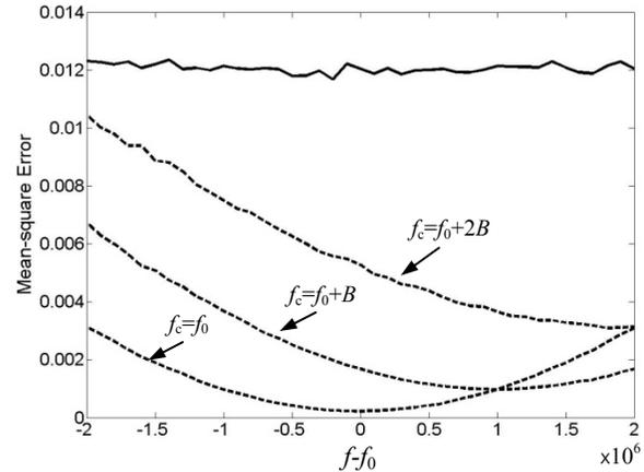
Fig. 2. Mean-square error in the estimated spectrum using regular stratified estimator (solid line) and IQ stratified estimator (dashed lines) with different  $f_c$  with  $N = 20$
