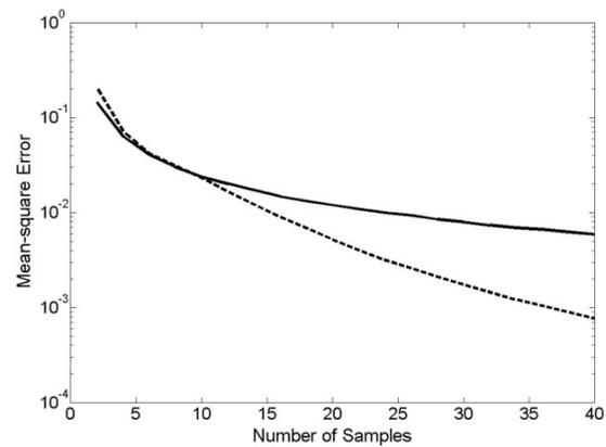
Fig. 3. Mean-square error in the estimated spectrum using regular stratified estimator (solid line) and IQ stratified estimator (dashed line) at frequency point  $f = 10^9$  Hz
