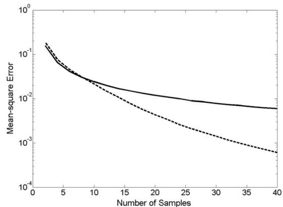
Fig. 4. Mean-square error in the estimated spectrum using regular stratified estimator (solid line) and IQ stratified estimator (dashed line) at frequency point  $f = 10^9 + B / 2 = 1.0005 \times 10^9$  Hz
