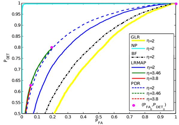
Figure 1: ROC of the NP, GLR, BF, LRMAP and PDR detectors. The NP, GLR and the BF tests are shown only for  $\eta = 2$ . At fixed  $\eta$ , the maximal extension in  $P_{FA}$  of the ROC curve of the PDR and LRMAP tests can be computed analytically through (4) and (5) (magenta points). These points correspond to set  $\gamma = 0$ , in which case the two tests become equivalent.
