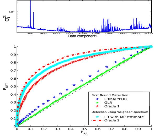
Figure 4: Top : Example of noise variances for a MUSE spectrum. Bottom : compared ROC by considering contiguous spectra as independent ("First Round Detection") and by exploiting spatial dependencies ("Using neighbor spectrum").
