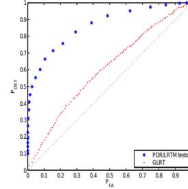
(c) ROC of PDR/LRMAP vs GLR at fixed  $SNR = -19.3$ dB.
