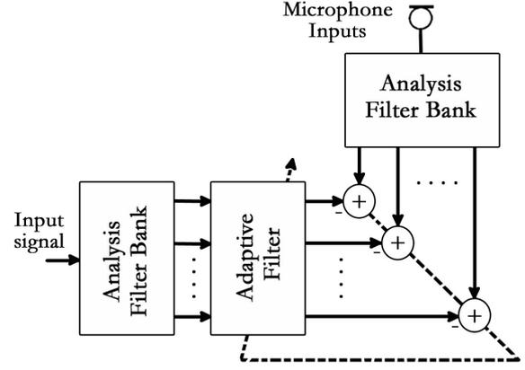
Figure 2: Scheme for the impulse response identification: for each microphone, the adaptive filter is composed of  $M$  weights  $H_n(m)$ .
