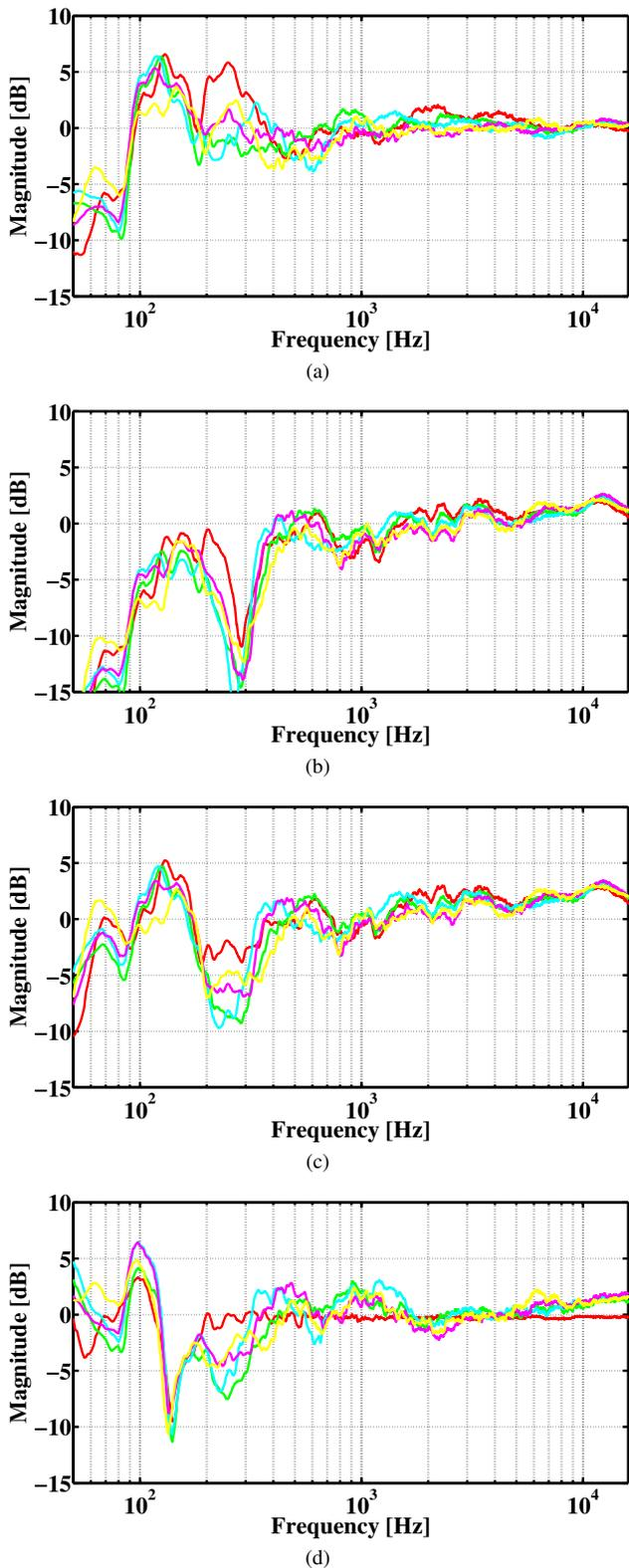
Figure 10: Room magnitude response after equalization. (a) Proposed method. (b) Method of [6]. (c) Method of [8]. (d) Method of [18].
