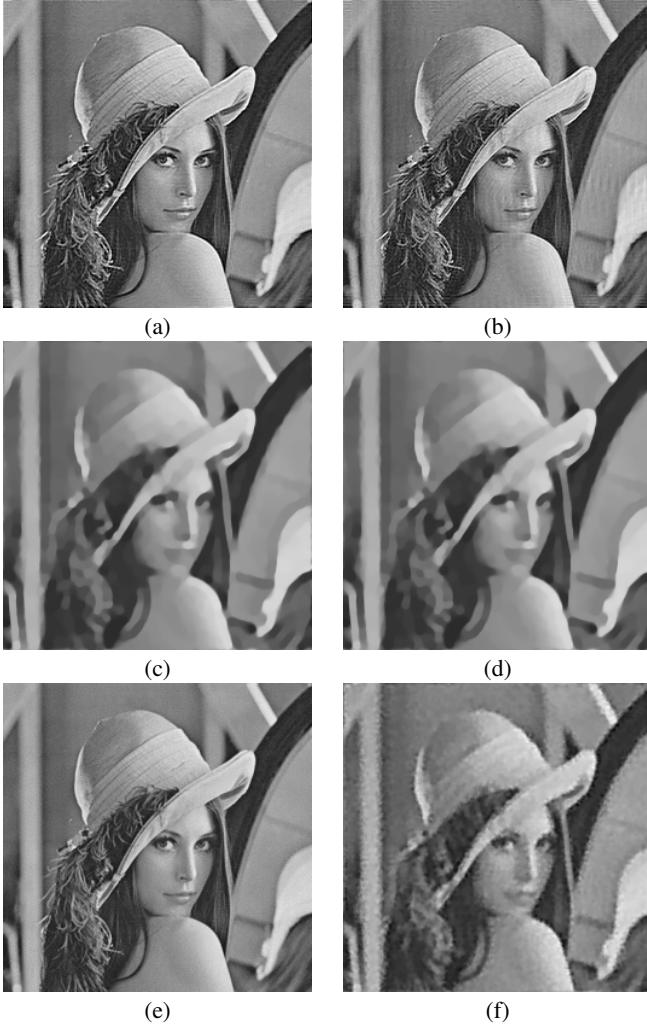
Figure 2: Restorations of the Lena image blurred with an out-of-focus blur with radius 4, and BSNR = 60 dB with (a) TV1 , (b) TV2 , and BSNR = 20 dB with (c) TV1 and (d) TV2 . The non-blind restoration results by TV1-NB are shown in (e) for BSNR = 60 dB and (f) for BSNR = 20dB.
