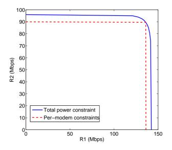
Figure 2: Rate region of BC-OSB in a VDSL2 system
