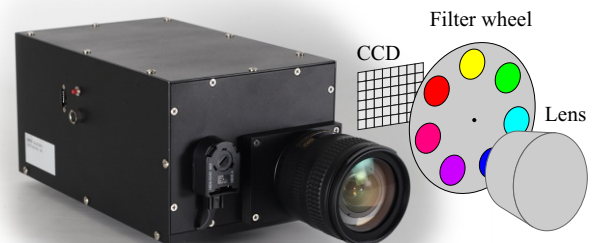
Figure 1: Our multispectral camera, using 7 optical filters. Its internal configuration is sketched.
