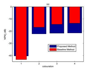
Figure 4: Performance of averaged (6 speech sets)  $NPM_f$  measures of: 4 different reverberation times for varying colouration.
