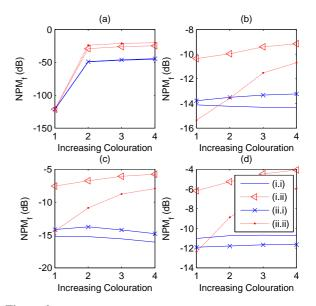
Figure 6: *Combined*  $NPM_f$  measure across (i.i) different speakers-Proposed method, (i.ii) different speakers-Baseline method, (ii.i) different utterance-Proposed method, (ii.ii) different utterance-Baseline method for different reverberation times (a)(b)(c)(d) and different colouration.
