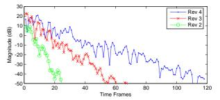
Figure 1: Example of the linearity of reverberation decays for frequency bin 50 for three different reverberation lengths.
