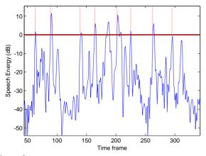
Figure 2: Example of the find onset algorithm for a particular frequency bin. Red dash spikes indicates an acceptable onset detected.
