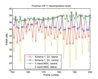
Figure 11: Central and lateral PSNR variation from the 150th to the 200th frame of the Foreman sequence (CIF, 30 Hz) at 1225 kBit/s.
