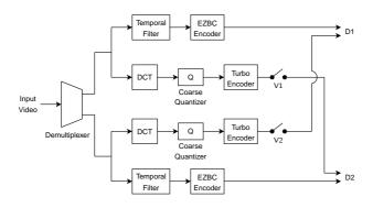
Figure 1: Implementation of the systematic lossy description encoder in pixel domain.
