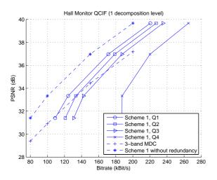
Figure 7: Central distortions of Scheme 1 compared with the 3-band MDC codec (Hall Monitor QCIF sequence, 15 Hz).
