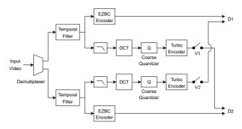
Figure 4: Implementation of the systematic lossy description encoder in MCTF domain.
