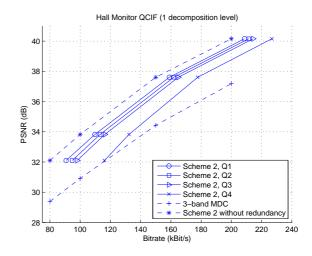
Figure 12: Central distortions of Scheme 2 compared with the 3band MDC codec (Hall Monitor QCIF sequence, 15 Hz).
