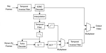
Figure 5: Implementation of the systematic lossy description side decoder in MCTF domain.
