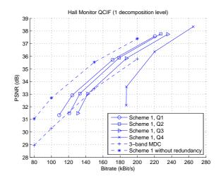
Figure 8: Lateral distortions of Scheme 1 compared with the 3-band MDC codec (Hall Monitor QCIF sequence, 15 Hz).
