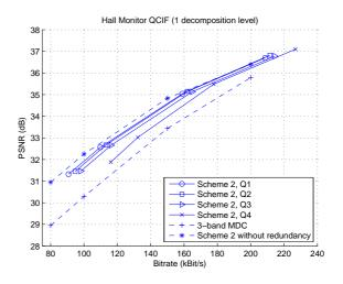
Figure 13: Lateral distortions of Scheme 2 compared with the 3band MDC codec (Hall Monitor QCIF sequence, 15 Hz).
