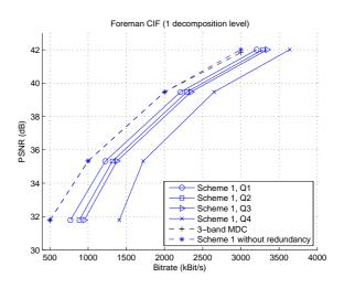
Figure 9: Central distortions of Scheme 1 compared with the 3-band MDC codec (Foreman CIF sequence, 30 Hz).
