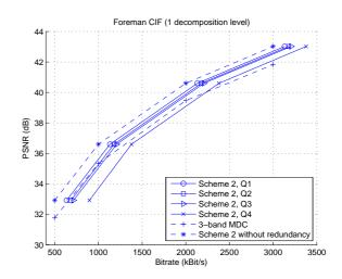
Figure 14: Central distortions of Scheme 2 compared with the 3band MDC codec (Foreman CIF sequence, 30 Hz).
