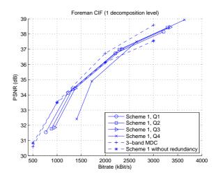
Figure 10: Lateral distortions of Scheme 1 compared with the 3band MDC codec (Foreman CIF sequence, 30 Hz).
