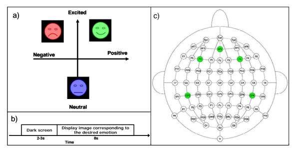
Figure 1 - (a) 2D emotions representation in the valence-arousal space, with indication of the three emotion classes considered in this study together with the visual symbol used to prime the participants. (b) Chronology of one trial in the emotional recall protocol. (c) Schematic representation of electrodes positions on the scalp for the Biosemi Active Two with 64 channel EEG and two references (CMS and DRL); the five channels selected by SL as the representative set are marked in green color.
