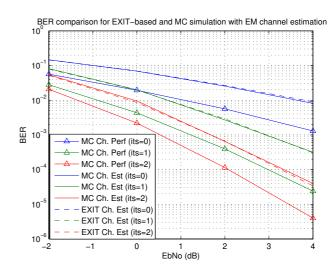
Figure 5: Comparison of EXIT fuction-based and MC simulation with soft decision-directed EM channel estimation and an initial  $4 \times 8$  training matrix.
