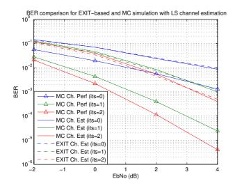
Figure 3: Comparison of EXIT fuction-based and MC simulation with LS channel estimation and a  $4 \times 8$  training matrix.
