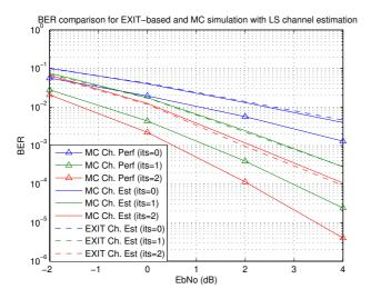
Figure 4: Comparison of EXIT fuction-based and MC simulation with LS channel estimation and a  $4 \times 16$  training matrix.
