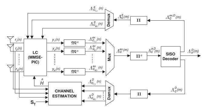
Figure 2: Diagram of a generic interference cancelation-based iterative MIMO receiver with channel estimation.
