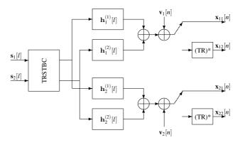
Figure 1: Data Model for a 2x2 TRSTBC system
