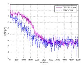
Figure 4: Mean square error curves for STBC-CMA and TRSTBC-CMA, SNR = 20dB.
