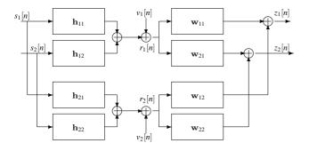
Figure 2: Channels and equalizers for a 2-by-2 MIMO system.
