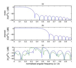
Figure 5: Magnitude responses of (a) lowpass noise (b) lowpass channel (c) *N* selected subband filters of the precoder for our OSFB disign. K = 8, N = 2 filters.
