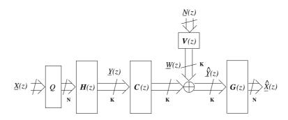
Figure 1: General model of the proposed OSFBs channel coding system.
