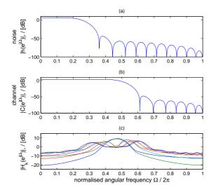
Figure 4: Magnitude responses of (a) lowpass noise (b) lowpass channel (c) N selected subband filters of the precoder for Mertins' design. K = 32, N = 8 filters.
