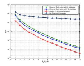
Figure 2: BER versus SNR for 4 different receivers.
