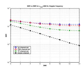
Figure 3: BER versus SNR for the two-step estimation in [4].
