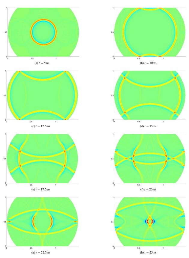
Figure 3: Simulation of the wave equation for the irregular domain from Fig. 1. The model is excited in the center with a band-limited Gaussian impulse and Neumann boundary conditions are applied, resulting in perfectly reflecting walls. The snapshots are taken at several time instances *t*, demonstrating the correct behavior of the block based model.
