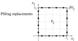
Figure 2: Spatial sampling at the boundary of region  $V_2$ . The sampling points  $\vec{x}_v$  are denoted by the black dots •.
