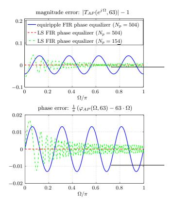
Figure 3: Approximation error for the desired transfer function of Eq. (15) obtained by phase equalization of an allpass chain of length L=63 (a=0.4) with phase equalizers of filter degree  $N_p$ .
