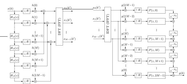
Figure 1: Polyphase network implementation of the allpass transformed DFT analysis filter-bank with downsampling and  $L=2\,M-1$ .
