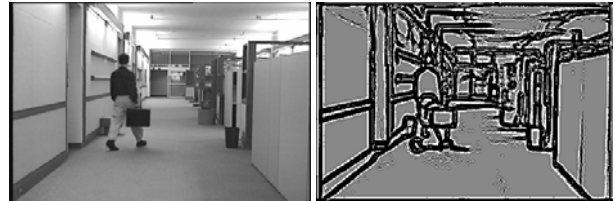
Fig.2 The map image \mathbf{M}(\mathbf{s},t) (right) for an original image (left). The map image contains the number that the mean shift converged to each pixel position. ( black : zero number of convergence, indicating pixels on image edges; white : high number of convergence, indicating pixels next to edges; gray : median number of convergence, indicating pixels in smooth areas).
