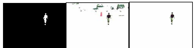
Fig.5 Example of detected moving object for the ‘car parking’ sequences (frame #66-67). Left : optical flow-based candidate regions; Middle : the 4 th order moment-based candidate regions. Right : detected moving regions after fusion.
