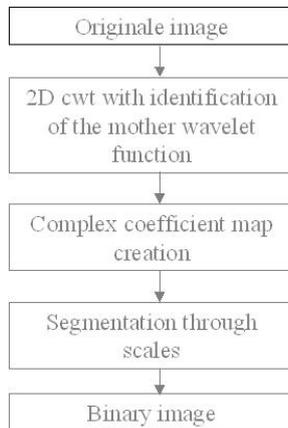
Figure 2: scheme of the image processing method proposed for pavement crack detection
