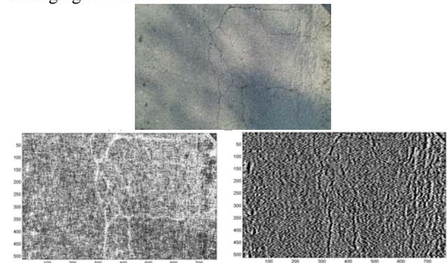
Figure 6: example of modulus and phase maps at scale 4
