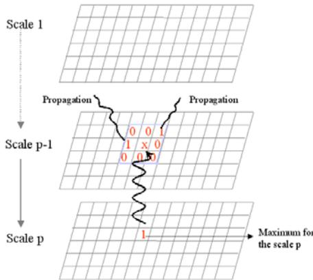
Figure 8: maxima propagation through scales
