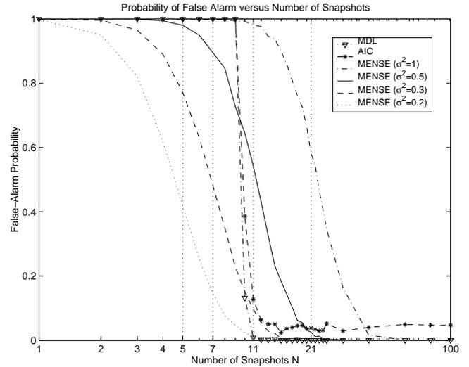
Figure 3. Probability of false alarm versus the number of snapshots for several noise variances for Example 3 (vertical dotted line: detection threshold;  $M = 10$ , and  $p = 0$ ).
