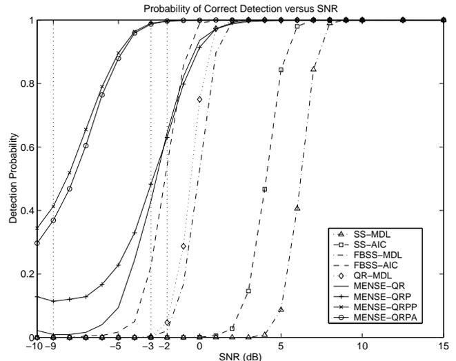
Figure 1. Probability of correct detection versus the SNR for Example 1 (vertical dotted line: detection threshold;  $N = 64$ ,  $M = 10$ , and  $p = 2$ ).
