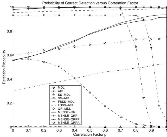
Figure 2. Probability of correct detection versus the correlation factor for Example 2 (SNR = 0dB,  $N = 64$ ,  $M = 10$ , and  $p = 2$ ).
