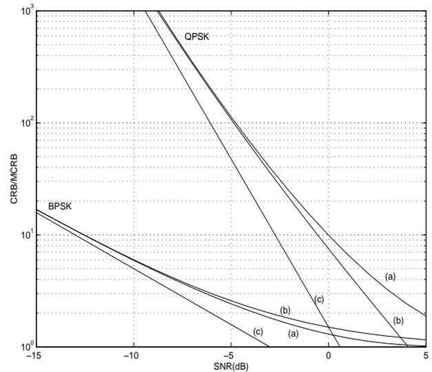
Fig.1 Ratio  $\text{CRB}(v)/\text{MCRB}(v) = \text{CRB}(\phi)/\text{MCRB}(\phi)$  at low SNR: (a) exact value given by (3), (4), (b) approximate value given by (7), (8), (c) approximate value given in [4].
