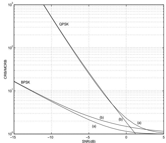
Fig.2 Ratio  $\text{CRB}(a)/\text{MCRB}(a)$  at low SNR: (a) exact value given by (5), (b) approximate value given by (9).
