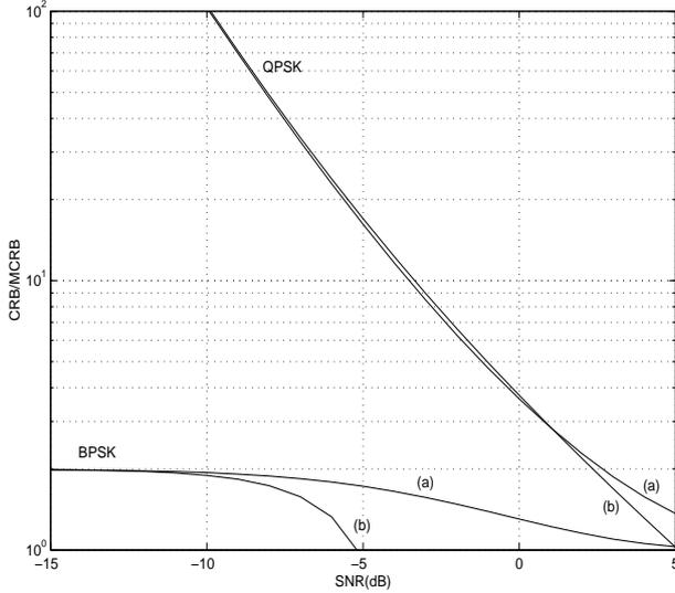
Fig.3 Ratio CRB( $\sigma$ )/MCRB( $\sigma$ ) at low SNR: (a) exact value given by (6), (b) approximate value given by (10).
