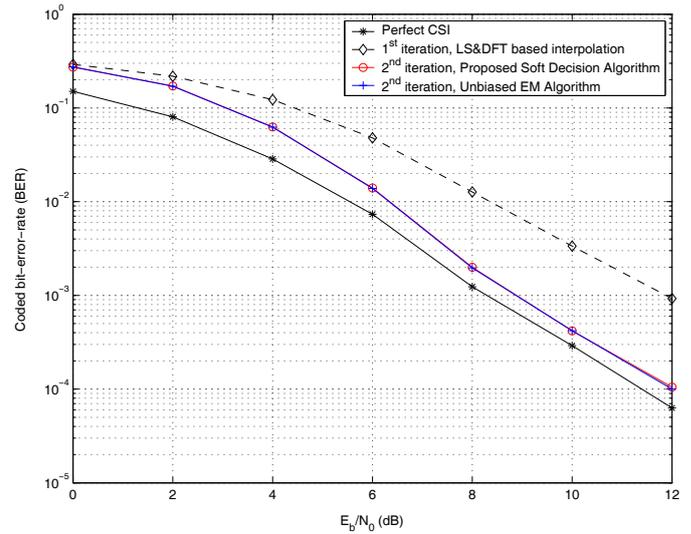
Figure 5: The BER performance of coded OFDM system
