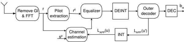
Figure 3: The receiver structure of coded OFDM system
