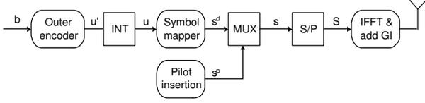
Figure 1: The transmitter structure of coded OFDM system
