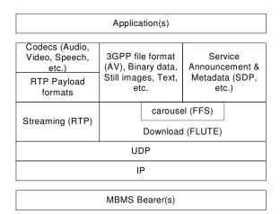
Figure 2 The MBMS Protocol Stack
