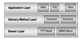
Figure 1 Functional Layers of MBMS
