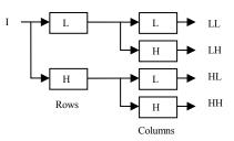
Figure 1. Illustration of discrete wavelet frame decomposition with lowpass (L) and highpass (H) filters. The input image is decomposed into four subbands.
