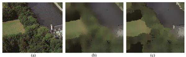
(a) (b) (c) Figure 4. The comparison of filtering results. (a) Original image. (b) Mean shift filtering result. (c) Texture supported filtering result. Note that the region boundaries are well-separated.
