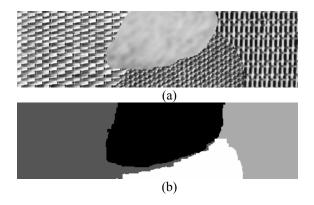
Figure 3. Illustration of classifying different textured regions. (a) A textured image containing vertical, horizontal, smooth and complex textures. (b) Classification result using DWF decomposition with median energy in a 15x15 local window.
