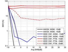
Figure 3 – BER performance for single user system – AWGN-CM1 channels - Time-hopping was not used.- Detector threshold = 16dB
