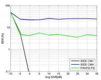
Figure 6 – BER performance for single user system- CM1, CM4 and PANFD radio channels with the receiver using the early-late synchronisation loop - without time-hopping - a relative detector threshold of -16dB.
