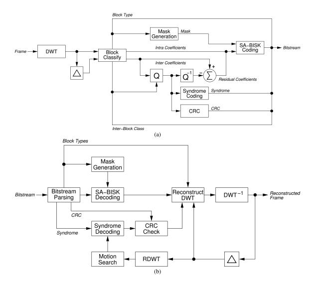
Figure 1: Block diagram of the WSC system, (a) encoder, (b) decoder.  $\Delta$  indicates a frame delay; Q indicates uniform scalar quantization.
