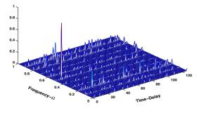
Figure 2: Spreading function of user 2 in multiuser communication channel (uplink) of 6 users.
