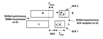
Figure 1: Time-offset SDMA slot for two users.
