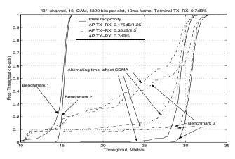
Figure 6: Throughput performance for two users and threeantenna AP in the "D"-channel 5.2 GHz environment.
