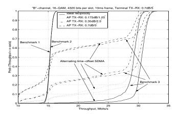
Figure 4: Throughput performance for two users and twoantenna AP in the "B"-channel 2.4 GHz environment.
