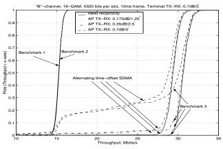
Figure 5: Throughput performance for two users and threeantenna AP in the "B"-channel 2.4 GHz environment.
